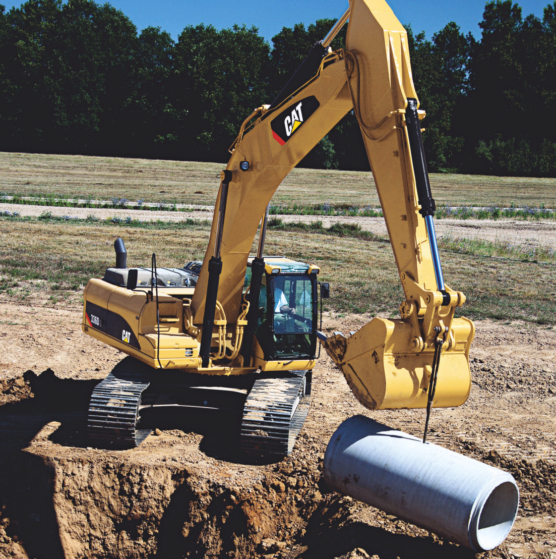
Shown here lifting concrete, the Caterpillar 336D L crawler excavator represents a model designation change. Formerly the 330D, the 336D L now weighs in, depending on configuration, at either side of the 80,000-pound mark. It is classified as the largest “medium” excavator by Caterpillar.
