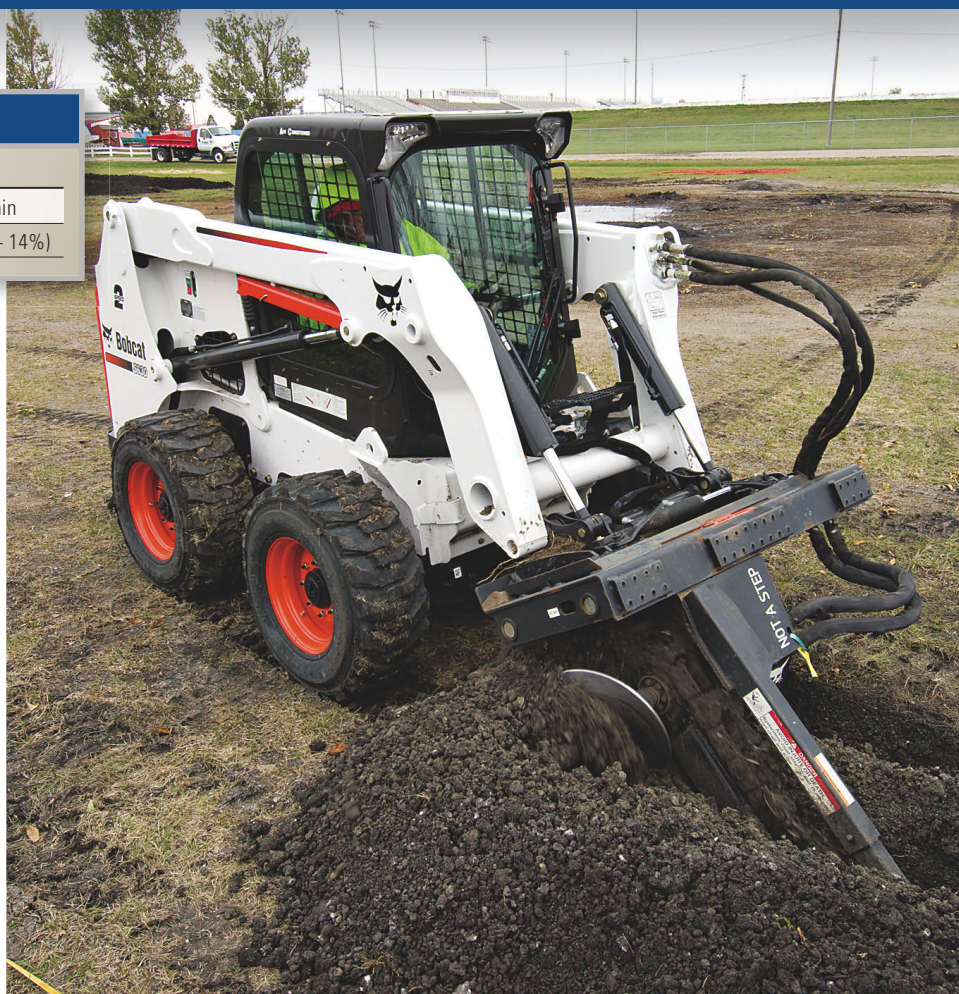
Operators pulled 100-foot trenches with a high-flow trencher on each loader. Improved hydraulic efficiency and instruments helped the S630 overcome its high-flow disadvantage.
